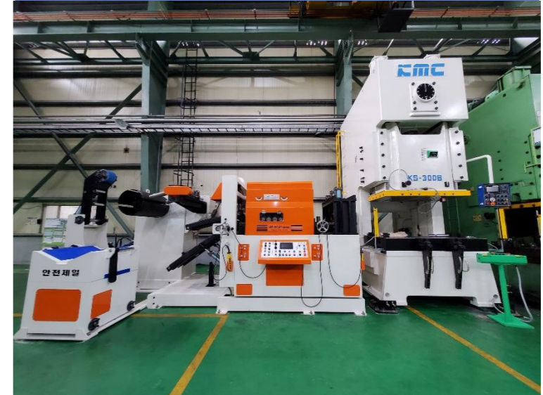
300TON PRESS & COIL FEEDER
